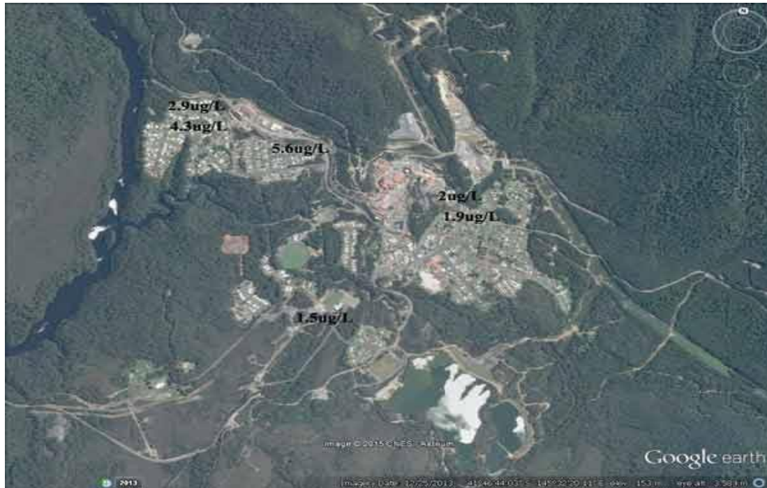
Rough location guide for Rosebery showing average levels of lead detected between July 2013 - June 2014. Note higher levels in north west of town. Huon Crst averaged 2.9µg/L, Blackwood Street 4.3µg/L, Howard St 5.6µg/L. Rear of hospital samples were taken between Jan 2014 and June 2015 and averaged 2µg/L.
